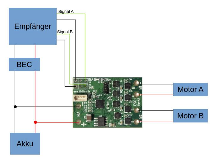
Input channel A controls motor A and input channel B controls motor B. For "Differential" and "Chain" modes, channel A must be the throttle channel and channel B the steering channel.
